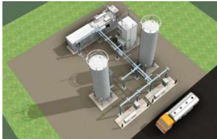
Figure 16. Cryotec's LNG E-LIN plant layout, capacity 12 TPD [Cryotec 2014].
