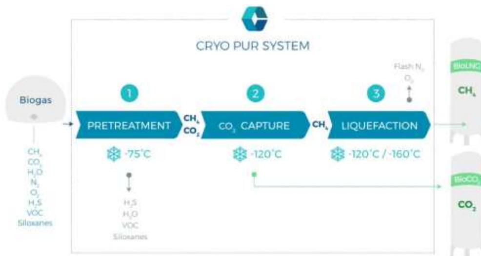
Figure 17. Integrated upgrading and liquefaction based on cryogenic upgrading [Cryo Pur 2020].
